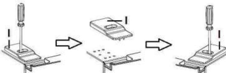
13. Lift the fridge door and remove it carefully (s. fig. below). Place the fridge door on a smooth surface with the external cladding facing up.
