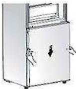
28. Align the middle door hinge (J) to the prepared holes on the left side of the appliance properly; s. fig. below (it may be necessary to turn the middle hinge through 180° to align it to the prepared holes properly -depending on model-). While doing so, insert the hinge pin of the middle door hinge into the top hinge hole of the freezer door. Screw the hinge tightly.
