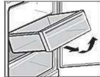
💡 Any of the freezer drawers can be removed and reinserted for cleaning as shown above.<sup>21</sup>
