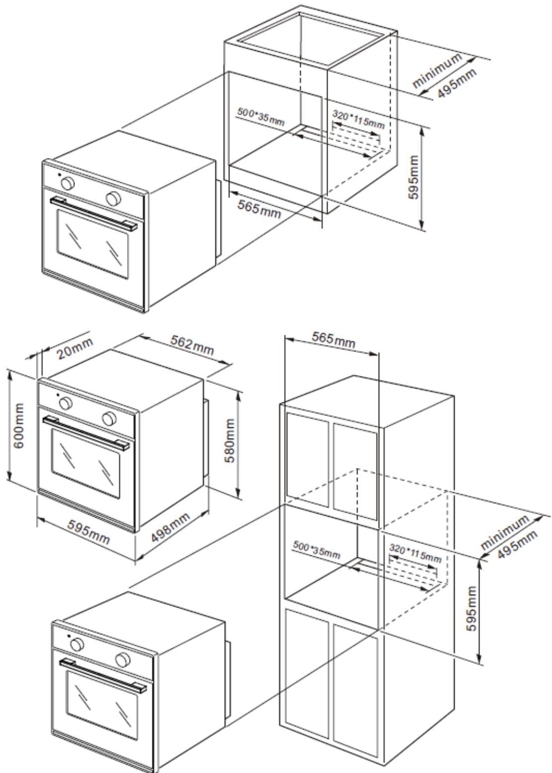
**FIG. 2: HOW TO FIX THE OVEN**
