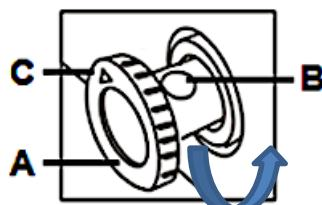
11. Push the water drain screw (A) back into the appliance carefully and properly (s. fig. below, black arrow).
