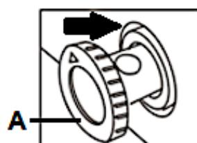
12. Reinstall the **water drain plug inside** the freezer (s. fig. below, black arrow)!
