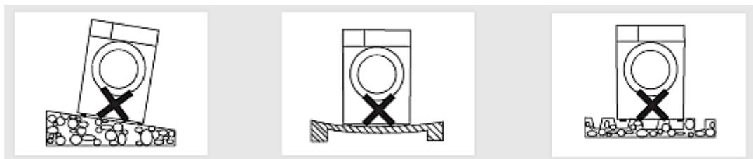
12. If you install the appliance on a wooden floor, you must also place it on a plywood panel (60.00\*60.00 cm) **at least** 3.00 cm thick to distribute the weight of the appliance. Fix and secure the plywood panel properly to the wooden floor.
