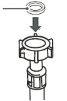
2. Attach the **straight** end of the water inlet hose to the appropriate water connection (s. fig. on the right).
