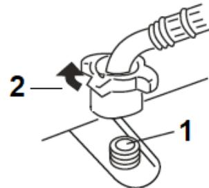
**NOTICE!** Do not overtighten the water inlet hose. Overtightening of the water inlet hose can damage the valves.
