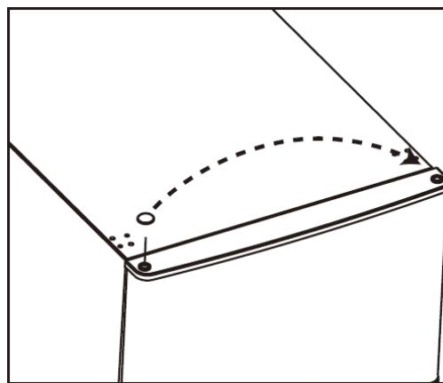
8. Lift the door and remove it carefully (s. fig. below). Place the door on a smooth surface with the external cladding facing up.
