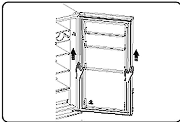
9. It is necessary to tilt the appliance backwards. Lean the appliance against a solid and immovable surface so it will not slip. **Do not** tilt the appliance more than  $45^\circ$ .
