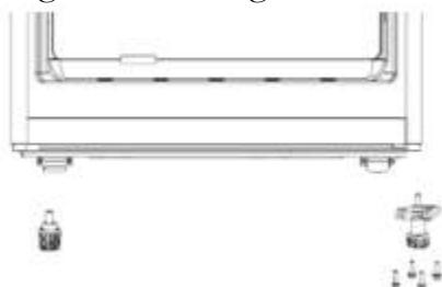
16. Unscrew feet (2) and then unscrew nut (3). Remove the hinge shaft (5) from the right hole (4) and insert it into the left hole. Tighten the nut and then tighten the feet.
