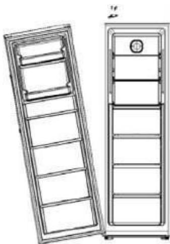
21. Open the door cover hole plug, remove the wiring harness terminal of the door, and connect with the wires in the cabinet one by one, then cover the hole plug.
