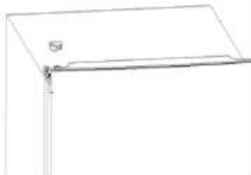
22. Install the supplied upper left hinge cover onto the cabinet after installing the cylindrical door switch and tighten the screw.
