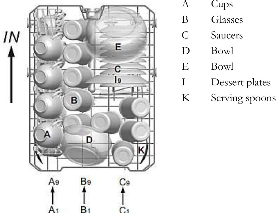
You can adjust the position of the upper dish rack to provide more room for large objects either in the lower or the upper rack. You adjust the upper rack by placing the relevant wheel-set in the rail. Put long items on the shelf so they will not impede the rotating spray arms. You can fold back the shelf if need be.
