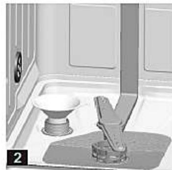
1. Remove the lower dish-rack and the lid of the water softener container.
